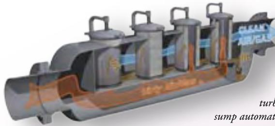
*R Series filters remove the solid particles and liquids from natural gas, vastly reducing or eliminating service to engines, turbines and other compressors, valves and meters. The new R100 filters permit horizontal service, vertical elements, turbulence baffled "Slug Catchers", & dual sump automated purge valves. Quick opening closures enable simple element change out.*
